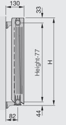
Connections: 4 x 1/2", suitable for bottom opposite ends (BOE), top bottom opposite ends (TBOE) or top bottom same end (TBSE). \*1/2" air vent Width excludes air vent  $\mathsf{F} = \mathsf{flow}$ R = return H = height W = widthAll dimensions in mm
