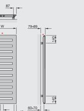
\*1/2" air vent Frame: 70mm x 39mm triangular tubes Flat tubes: 70mm x 8mm  $\mathsf{F} = \mathsf{flow}$ R = return H = height W = width All dimensions in mm
