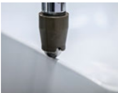
THE THIN-WALLED SAPHIRKERAMIK WAS TESTED FOR IMPACT RESISTANCE AT THE KERAMIK INSTITUT MEISSEN
