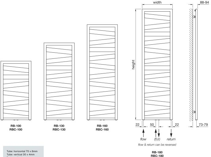
Tube: vertical 30 x 4mm D-shaped tubes All dimensions in mm
