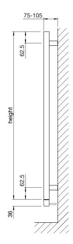
Tube: Horizontal Ø18mm Vertical 30mm x 30mm All dimensions in mm
