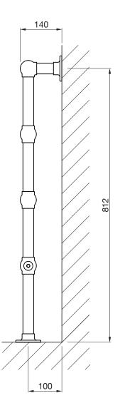
Tube: Horizontal Ø31.8mm Tube: Vertical Ø31.8mm All dimensions in mm
