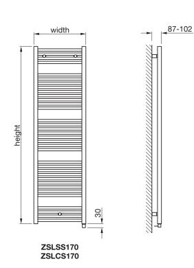
Tube: Horizontal Ø23mm Vertical Ø38mm All dimensions in mm
