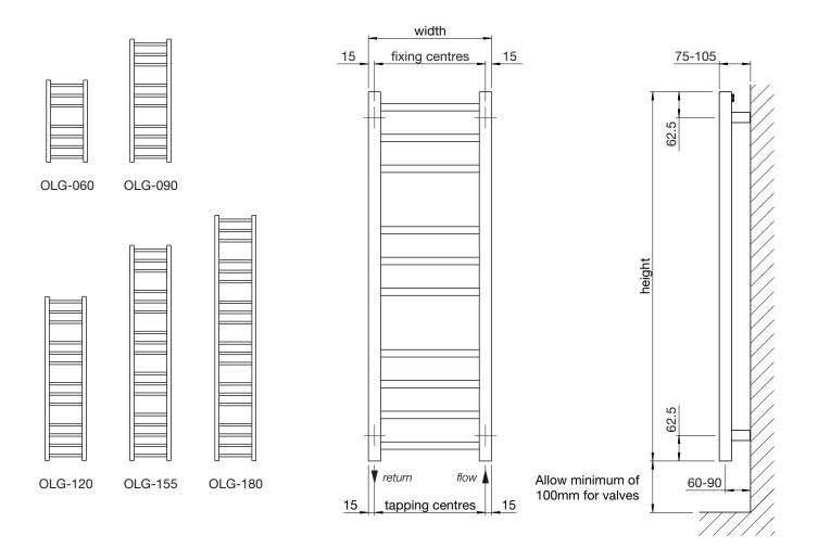
Tube: Horizontal Ø18mm Vertical 30mm x 30mm All dimensions in mm
