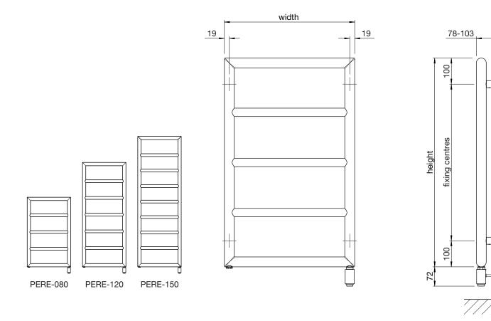
Tube: Horizontal Ø32mm Tube: Vertical Ø38mm All dimensions in mm
