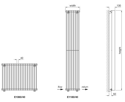
Tube: Horizontal Ø30mm Tube: Vertical 70mm x 8mm All dimensions in mm
