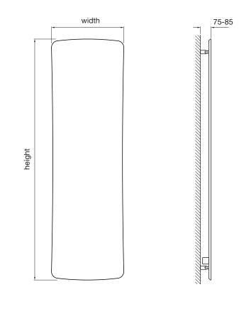
Available as both a central heating and electric radiator Projection from the wall to front face: 85mm Electric version controlled via radio frequency remote programmer
