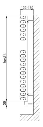
Tube: Horizontal Ø25mm Tube: Vertical Ø26mm All dimensions in mm
