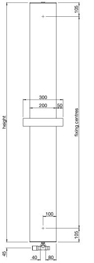
straight or angled valves are supplied with this radiator (see separate sheet for fitting instructions)
