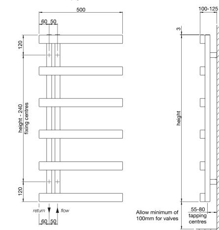
tiow ↓ return Radiator can be inverted and hung in this orientation
