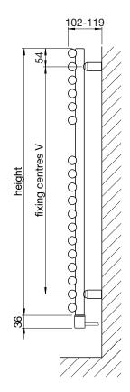
Tube: Horizontal Ø25mm Tube: Vertical Ø26mm All dimensions in mm
