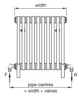
F = flow R = return Tube: Vertical Ø 25mm All dimensions in mm Manufacturing tolerance of +/-0.6mm per section
