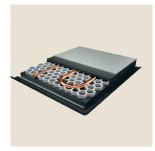
The aluminium honeycomb structure, with its meandering copper pipe, is filled with graphite, enabling heat to be distributed throughout the entire front of the radiator quickly and evenly. Suitable for all low temperature systems, heat pumps, condensing boilers, open or closed heating systems.
