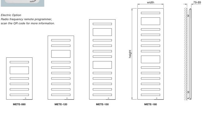
Frame: 70mm x 39mm triangular tubes Flat tubes: 70mm x 8mm All dimensions in mm
