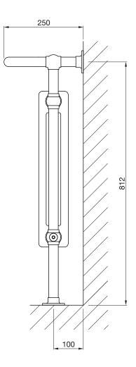
Tube: Horizontal Ø31.8mm Tube: Vertical Ø31.8mm All dimensions in mm
