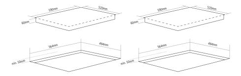
Induction hobs C950i & C901i: A minimum gap of 20mm is required beneath the hob fans, and a 4mm gap must be left under the worktop at the front of the hob for ventilation.
