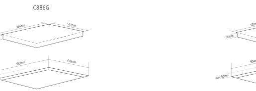
If installed without a gap in between, cut-out width = [no. of hobs - 1] x 288mm] + 268mm
