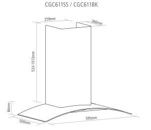
650mm space for electric hobs and 760mm space for gas hobs required from worktop to the mesh filter behind the centre glass panel. From the lowest point of the hood the distance required is 450mm for electric hobs and 550mm for gas hobs.
